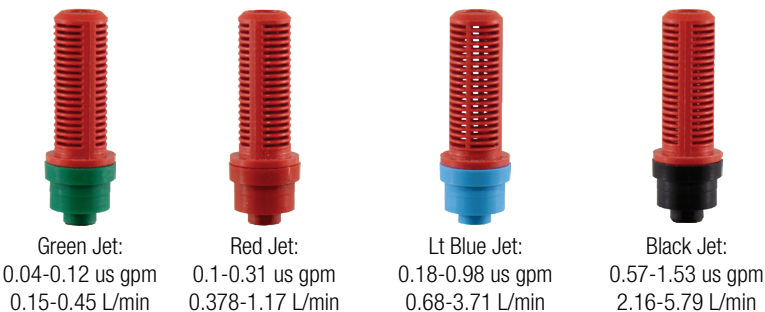
Figure 4. Flow Stabilizing Jets for measuring flow ranges
