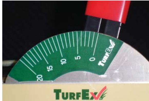
Now put a small amount of material in the spreader to determine the spread width of your product at the speed that you will be walking. To determine your ground speed measure the distance you cover in 1 minute and reference the chart below.
