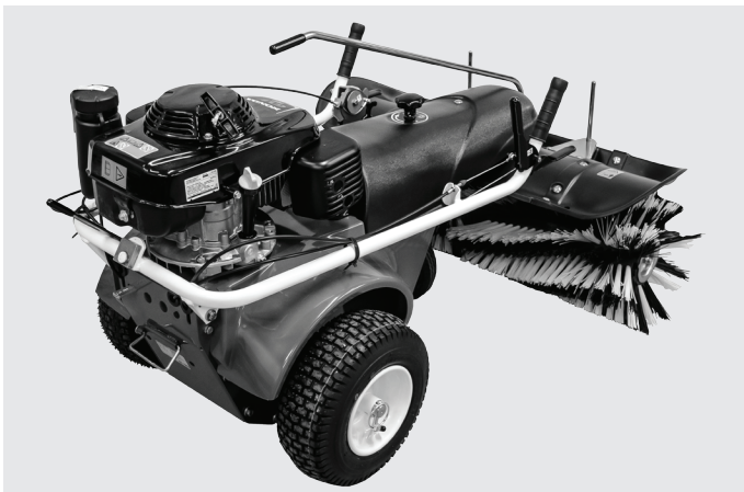
You can fold the handlebars fully forward to save space when storing or transporting.
