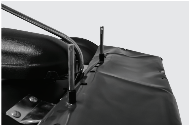
Slide the Debris Shield over the receiver bars.
