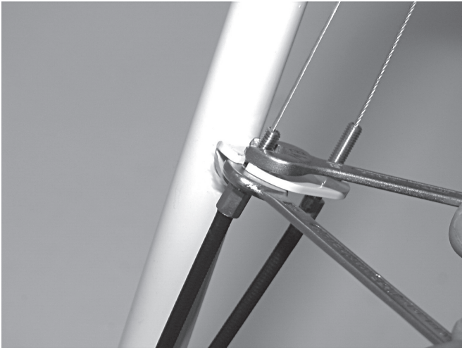
Loosen the top nut with a 10 mm wrench (about one turn).
