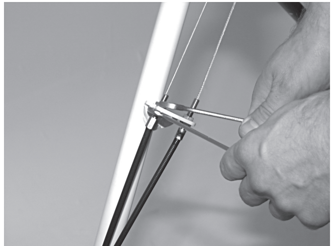
Tighten by turning the lower nut.
