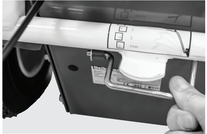
Push the 'lever lock' down (centered at the base of the handlebars).
