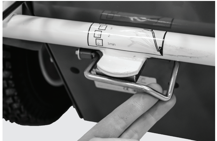
Tilt the handlebars back into position; push the 'lever lock' back in place to lock.
