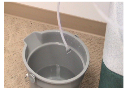
Place Chemical Feed Hose into Rinse Solution
