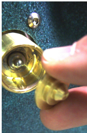
Place concave side of Spring Plate on top of piston.
