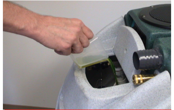
Add appropriate amount of chemical to water in solution tank
