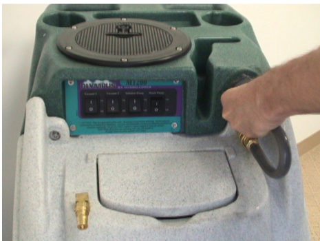
Place end of prime hose and use vacuum to prime the solution pump.
