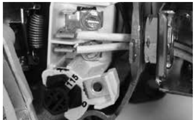
Figure 8: Voltage set to 115 V, Dial Type
