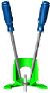
Figure 16 - Remove Mechanical Seal
