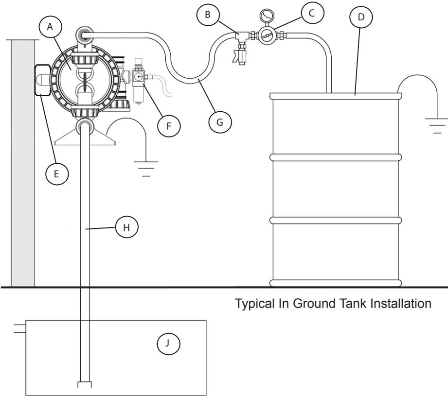
Typical In Ground Tank Installation
