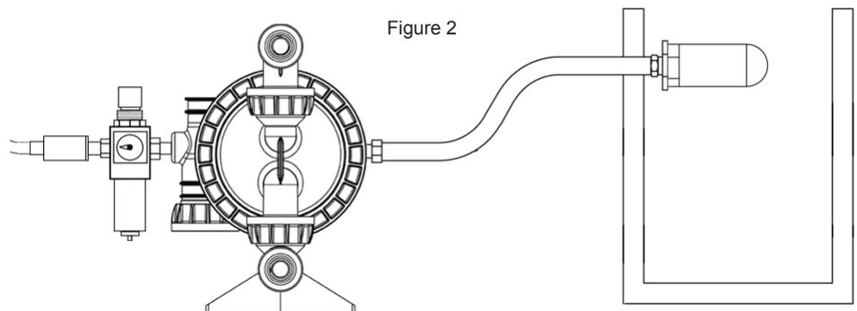
Install an electrically conductive air exhaust hose, connecting the muffer at the end. Minimum diameter for the hose is 3/8" ID. If the hose run will exceed 15', a larger diameter hose is required. Take care when routing the hose to avoid kinks and sharp bend that may restrict air flow.
