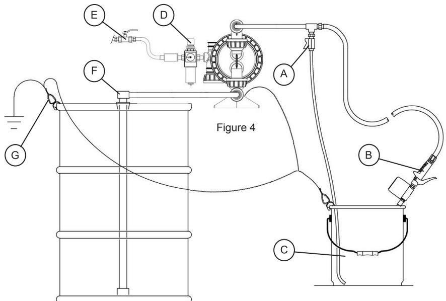
**⚠ WARNING** **WARNING! PROPER PUMP SHUTDOWN!** Diaphragm and seal life may be reduced if air pressure is applied to the pump motor during long periods when the pump is not being used. Installing a 3-way solenoid valve that automatically relieves pressure on the air motor when a metering cycle is complete prevents this from occurring.
