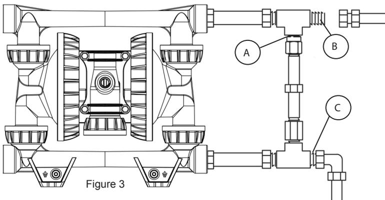
Some systems may require installation of a pressure relief valve at the pump outlet to prevent overpressurization, and possible rupture of the pump or hose (Figure 3).
