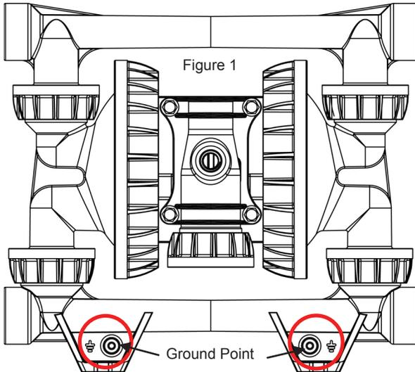
The SP100 pump can be grounded through the mounting feet, located on the inlet manifold (Figure 1). To reduce the risk of static spark, ground the pump and all other equipment located in the pumping area. Ground wires should be of proper size and installed per local and national electrical codes.
