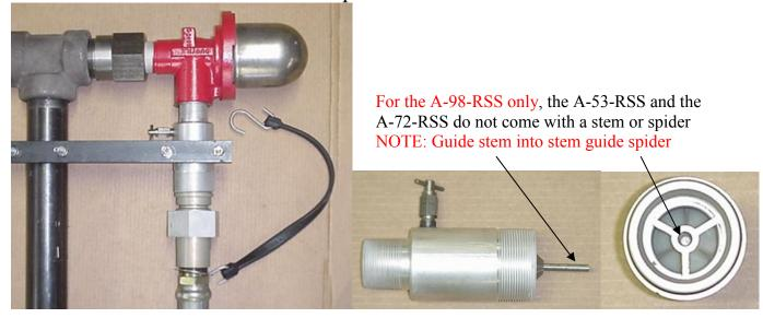
10. Then screw the RSS-NUT union nut onto the RSS-BODY inlet body and tighten firmly and pinch the bungee hook closed to prevent it from slipping off as shown in the picture below \*\*\*When tightening the union nut DO NOT PUT ANY WRENCH ON THE RSS-SHEAR, SHEAR BODY. This will cause the unit to prematurely brake.\*\*\*.
