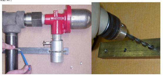
7. Cut off any excess material from the stabilizing bar as shown in the picture below.\*\*\*Make sure to leave at least 1" of material on the stabilizing bar.\*\*\*
