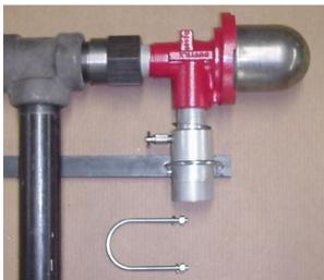
6. Mark and drill 2 = 11/32 holes for the accompanying u-bolt that will be used to attach the stabilizing bar to the riser piping as shown in the pictures below.
