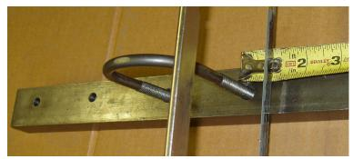
8. Install the Stabilizer bar with appropriate u-bolts, nuts and lock washers as shown in the picture below. \*\*\*Make sure to tighten bolts firmly.\*\*\*
