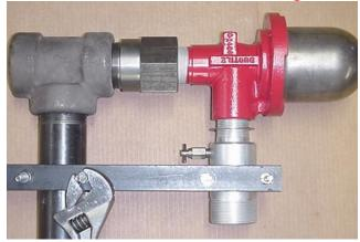
9. Attach the RSS-SHEAR shear body with the RSS-NUT union nut and hose assembly to the RSS-BODY inlet body by pushing the unit into RSS-BODY inlet body making sure both o-rings are completely inside the RSS-BODY inlet body. If you have the A-98-RSS make sure you guide the stem that protrudes from the RSS-BODY into the stem guide spider in the RSS-SHEAR as shown in the photo's below
