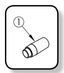
**Important:** The seal installation tool ① is required to install the shaft seal. This tool is included with the repair kit RK-BAC-75-M (40138). It prevents damage to the seal lips during installation over the splined shaft.
