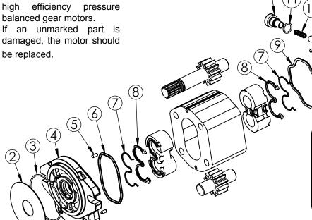
**Note:** The new seal kit (RK-BAC-75-M) may be used on all M Series motors without a case drain. See Product Update 19 for full details.
