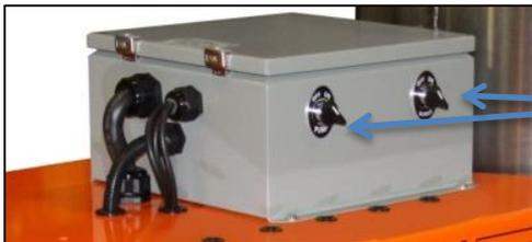
BURNER and PUMP Switches
