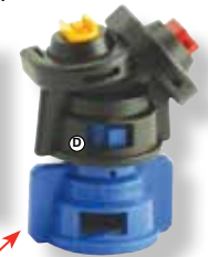
TADF-D / TACDF-D Dual Fan Nozzle (10° Forward & 50° Rearward) 40-80 PSI Range Best 110° Wide
