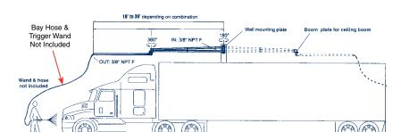
Whenever extended lengths and maximum flexibility are required, the wall boom extension is perfect for the job. Prime examples are truck wash bays, mining facilities, air craft maintenance and manufacturing plants. When combined correctly, a working radius of 39' is possible.
