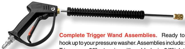
**Complete Trigger Wand Assemblies.** Ready to hook up to your pressure washer. Assemblies include: Trigger gun, 36" extension with molded grip, 3/8" inlet quick nipple, 1/4" quick coupler outlet. Rated to 8 GPM, 4000 PSI and 220° F. **Nozzles are not included.**
